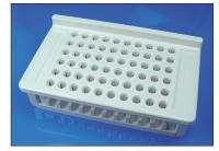
over a magnetic separation rack containing permanent magnets. The two piece design allows immunoassays to be set up, incubated and magnetically separated without removing the assay tubes from the test tube holder.
