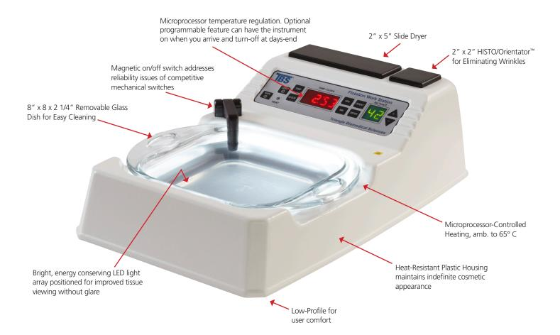
Flotation Work Station, microprocessor controlled with removable glass bowl w/built-in LED light array, 2" x 5" slide dryer and 2"x 2" HISTO/Orientator™, TUV/CE/FCC.
