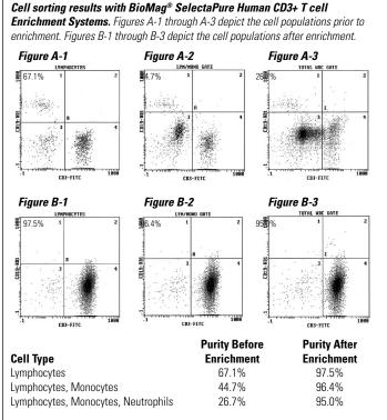
The BioMag® SelectaPure Human CD3+ T cell Enrichment System targets removal of CD19+, CD16+, CD14+, CD56+, CD11b+, and CD36+ cells. The particle to target cell ratio is 5.6.
